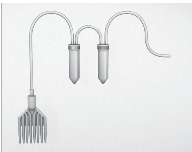
Figure 3–1: Schematic view of an assembled set up for vacuum-assisted emulsion breaking and bead recovery for Large Volume Emulsions
